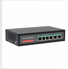
S-POE SW 1004 POE Switch 4 PORT 10/100 Mbps + 2 UPLINK PORT
